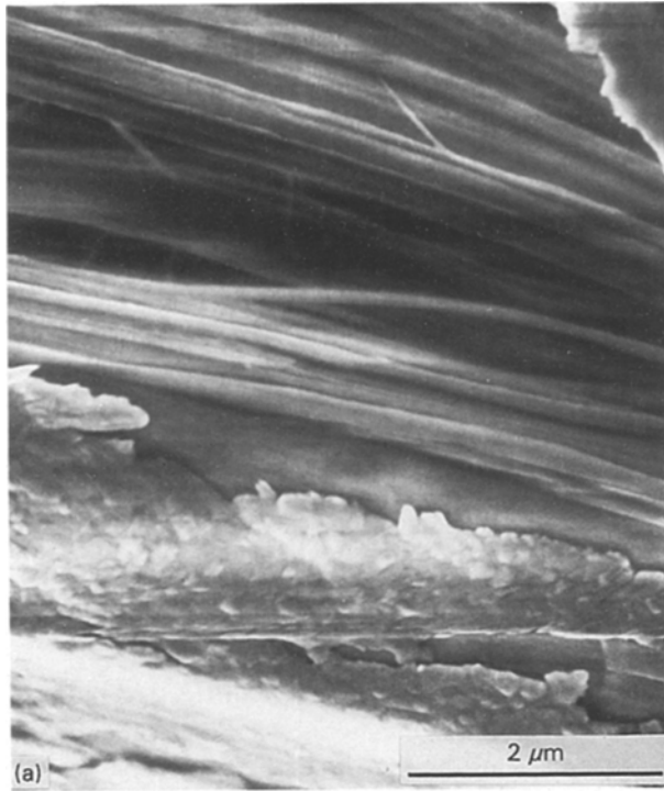
Figure 5 (a, b) High-resolution scanning electron micrographs of an aluminium-coated PBZT fibre.
